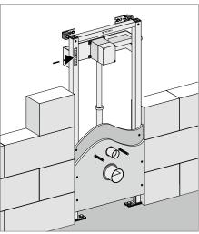
Mounted in front of a solid wall Masonry installation
