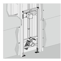
Mounted within a rail system Dry wall installation
